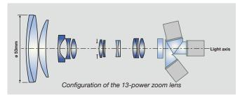
The wide-angle zoom lens that became so popular in the HVX200 Series has been downsized, lightened, and further widened in this 13X zoom lens. The new lens structure combines 13 lens elements in 10 groups, with 3 aspherical lenses. The diameter of the front lens element has been reduced from 67 to 53.2 mm, while still achieving a 28mm wide angle (35mm equivalent), the widest of the class.\*
